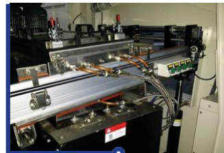
Nitrogen system for wave soldering
