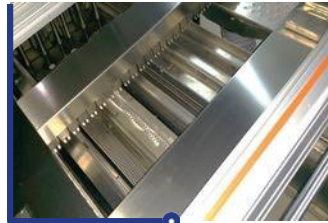
Dual wave solderpot (Full Ti-alloy)
